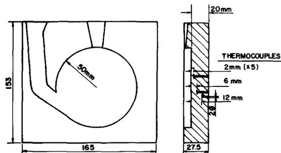
Figure 1 One half of the mould, showing the location of thermocouples.
