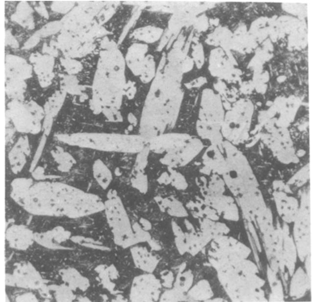
Figure 4 Needle-shaped  $\alpha$  grains of a casting made in a mould pre-heated to  $400^{\circ}\text{C}$ . Graphite coating thickness  $0.01\text{ mm}$  ( $\times 360$ ).
