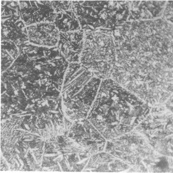
Figure 2 Aluminium bronze, water-cooled from the liquid-state. Nucleation of  $\alpha$  phase (white) at the grain boundaries; at the grain centre- $\beta$  phase. ( $\times 460$ ).
