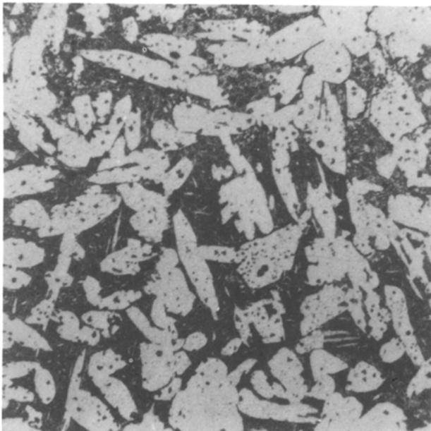
Figure 3 Needle-shaped  $\alpha$  grains of a casting made in a mould pre-heated to  $150^{\circ}\text{C}$ . Graphite coating thickness  $0.01\text{ mm}$  ( $\times 360$ ).
