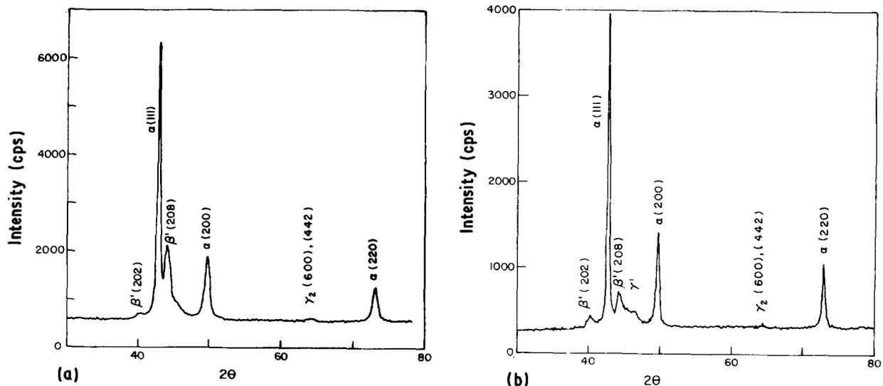
Figure 7 X-ray diffraction of aluminium bronze. (a) No formation of  $\gamma'$  when casting into cold mould. (b) Segregation of  $\gamma'$  when casting into hot mould followed by slow rate solidification.
