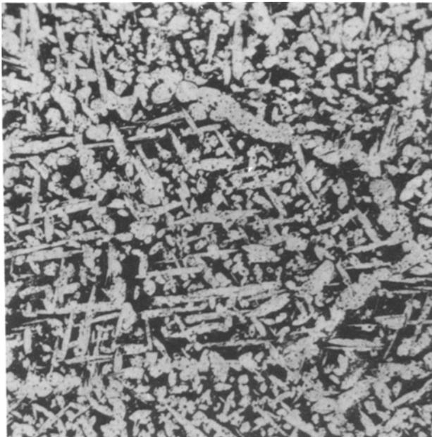
Figure 6 Needle-shaped  $\alpha$  grains with emphasized boundaries, in a casting made in a mould coated with graphite 0.10 mm thick ( $\times 230$ ).
