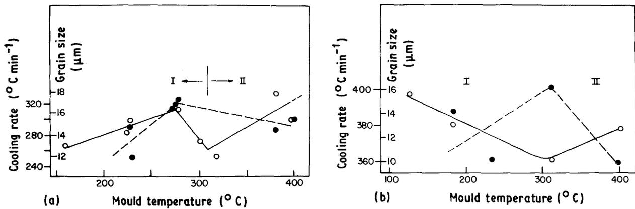
Figure 10 The interdependence of the cooling rate (●) and  $\alpha$  grain size (○) as a function of the pre-heating temperature of the mould. (a) Graphite coating thickness - 0.01 mm; (b) Graphite coating thickness - 0.10 mm.
