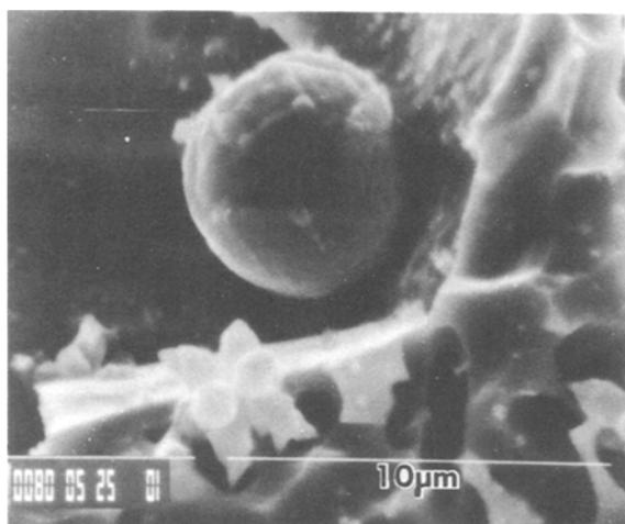
Figure 9 SEM image of a spherical iron particle (top) and a  $\text{Fe}_3\text{Al}$  precipitate in a grape-like structure (bottom).
