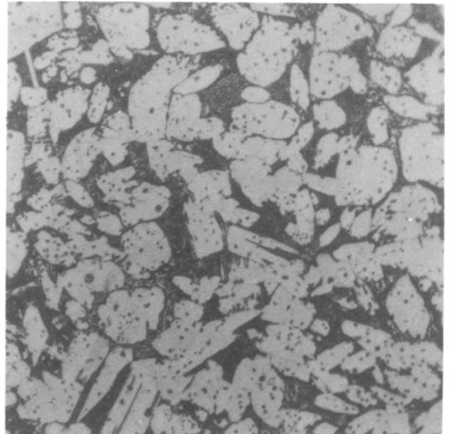
Figure 5 Highest cooling rate, spherical  $\alpha$  grains. Mould pre-heated to  $280^{\circ}\text{C}$ . Graphite coating thickness  $0.01\text{ mm}$  ( $\times 360$ ).
