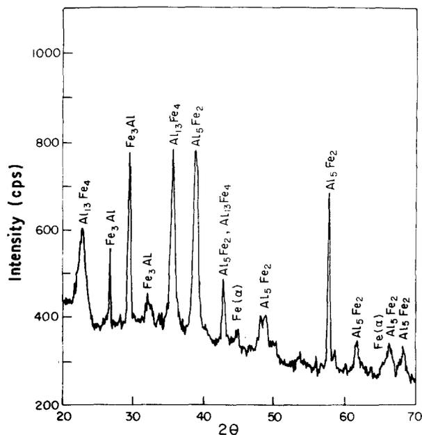
Figure 8 X-ray diffraction of the system Fe–Al after dissolution of the matrix and extraction of the powder.
